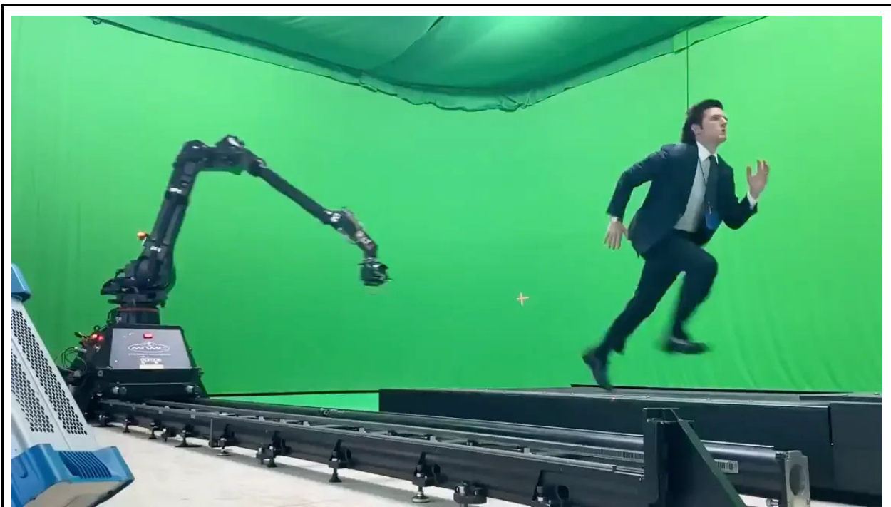
A BOLT robotic arm being used to create the running sequence in Severance (2025)
